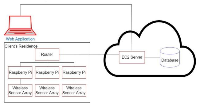
The planned design for the elderly individual's residence is in their kitchen. There will be arrays of sensors in cabinets and drawers. Each of these arrays connect through bluetooth low-energy to their predetermined Raspberry Pi. Once the information is received by the pi it is then transmitted to the cloud via the residence's router.
